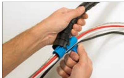
Place the HAT applicator tool in one end of the Helawrap cable cover.
