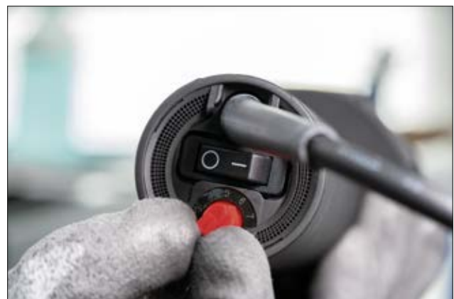
Adjusting H6100 operation temperature.
