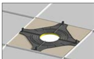
2. Cut the ceiling plate.
