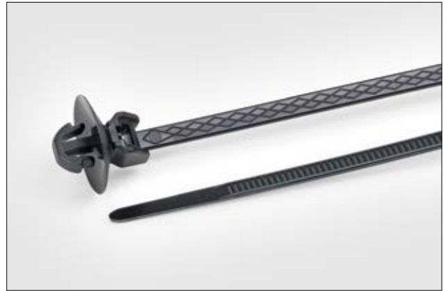
T30SOS-AS-SFT6.5x4E, 1 piece fixing tie with AntiSlip engraving and for a round hole 6.5 mm or a square hole 6.5x4 mm.
