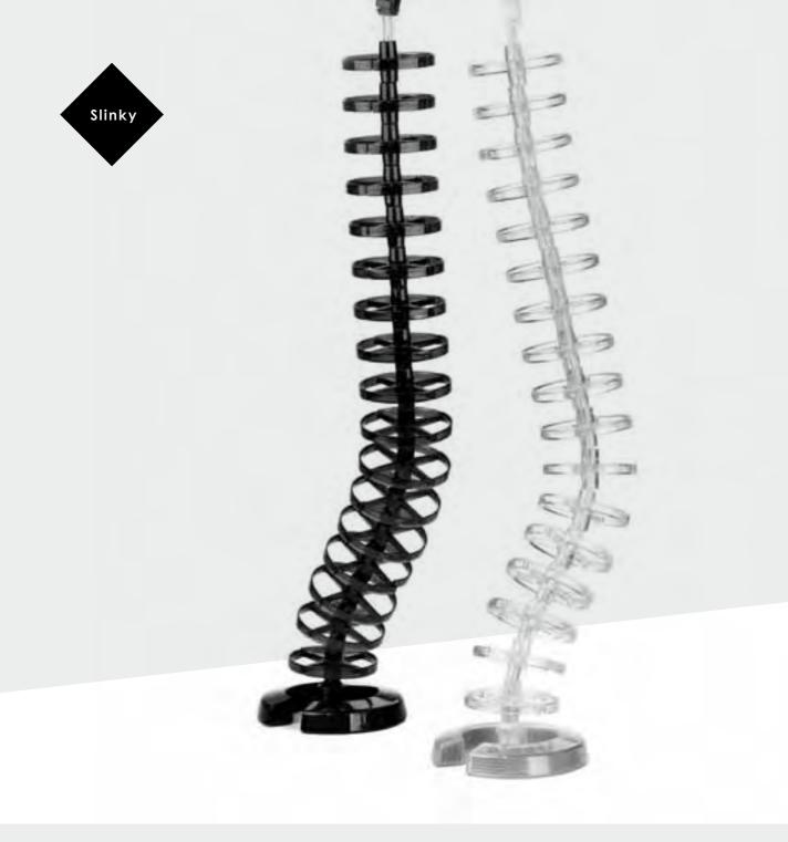
Slinky is a high-capacity cable management system of plastic vertebrae built around a flexible spine. Each vertebra has four separate compartments enabling power, data and voice cables to be separated. Slinky can easily be attached to the underside of the desk with a cast iron base anchoring it securely to the floor. **Product Code** Slinky - 800mm (31 1/2") WM3/001
